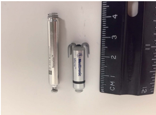
Figure 1. A Nanostim and a Micra pacemaker side by side.
