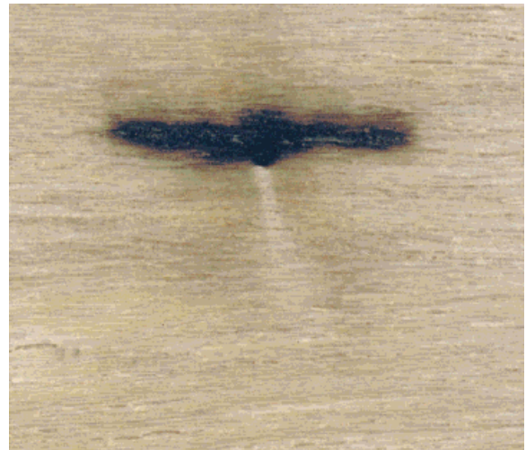
Figure 3. Evidence of significant heating at the tip of the copper wire as a consequence of finding the resonant length. [Color figure can be viewed in the online issue, which is available at www.interscience.wiley.com .]
