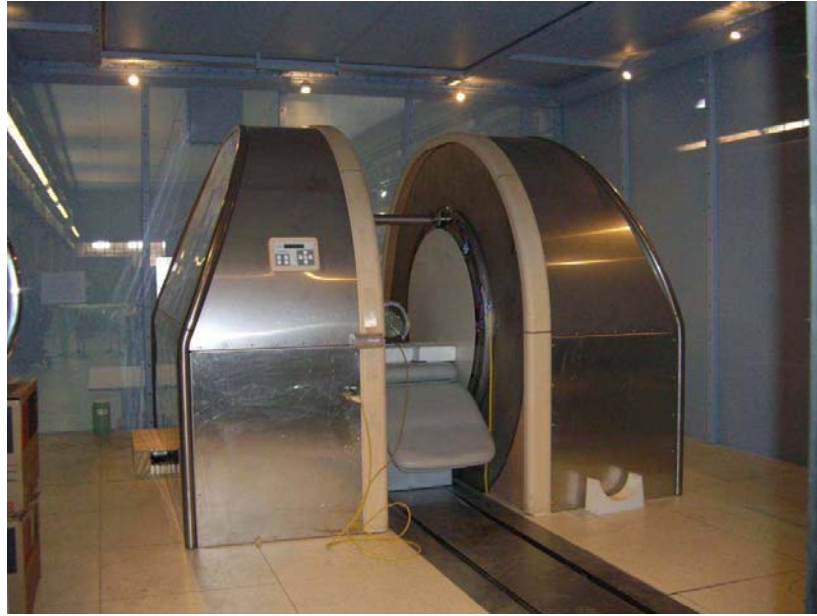
Figure 2.8: MgB_2 based, cryogen-free, open MRI magnet [235].
