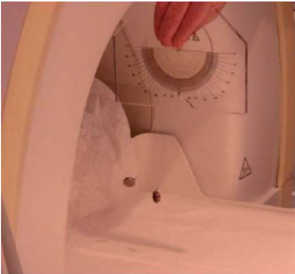
Fig. 3. Measurement of the deflection angle at 3 Tesla.
