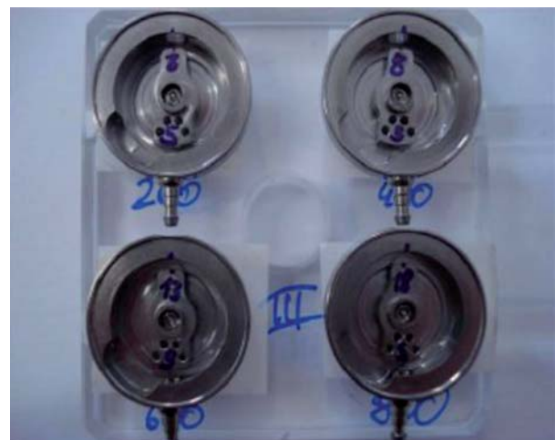
Fig. 2. The valves are bonded on a plastic frame for MRI investigation.
