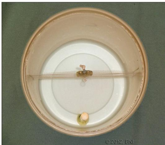
**Figure 3: Photograph demonstrating the artifact testing phantom with a shunt valve suspended in the center of the chamber for evaluation. During testing, the phantom is filled with gadolinium-doped saline [Used with permission from Barrow Neurological Institute]**
