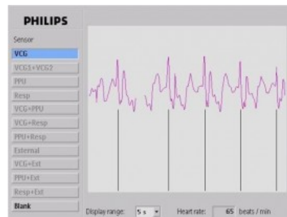
Figure 3b VCG at 3.0T inside magnet bore.
