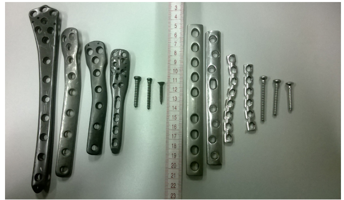
Fig. 1. Plates and screws used for displacement force test: titanium alloy materials (left) and stainless steel materials (right).
