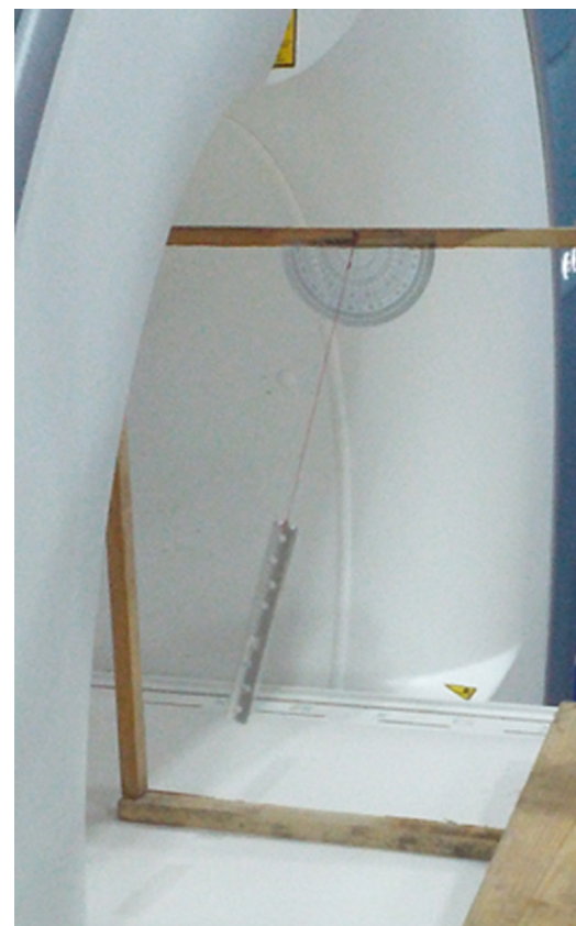
Fig. 2. An angel-measuring instrument which was self made: the plate was positioned in the area where the largest attraction force was produced.
