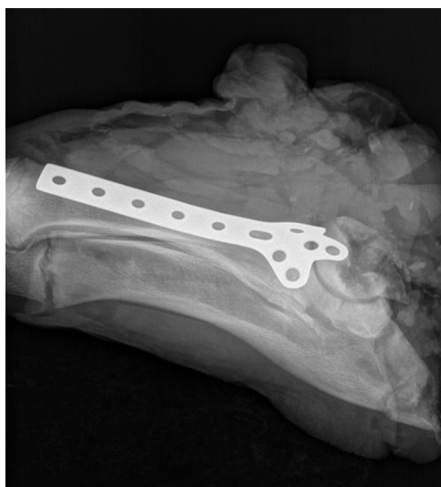
Fig. 4. Specimen for MRI-related heating test: a swine leg with plate implantation.
