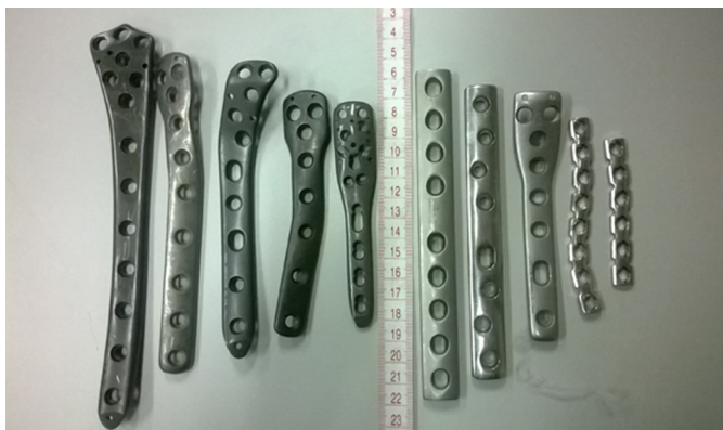
Fig. 3. Plates used for MRI-related heating test: titanium alloy materials (left) and stainless steel materials (right).
